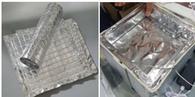
Figure 1. Vacuum insulation panel containing aerogel blankets.
