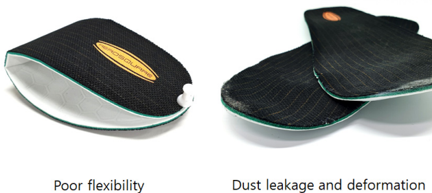
Figure 6. Durability problems after a long term use of aerogel blanket-based shoe insole prototypes.
