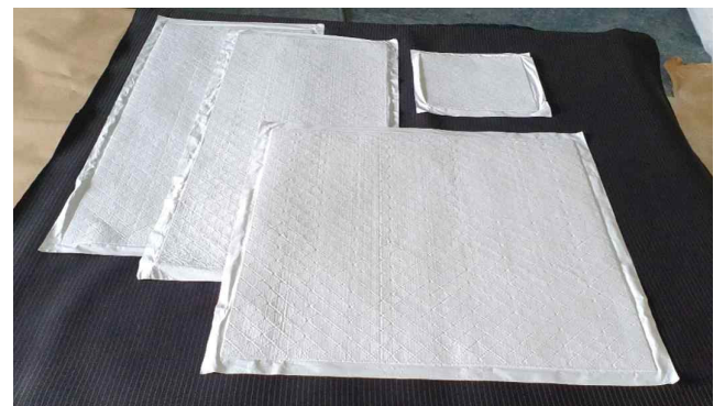
Figure 4. Multilayered aerogel blanket composite samples prepared for testing.
