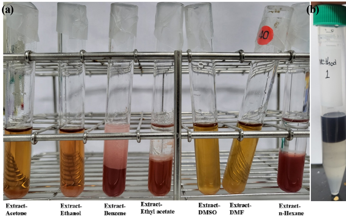
Figure 3. The effect of (a) various organic solvents and (b) polyethylene glycol-sodium citrate on the separation of pigments from grape skin extract.
