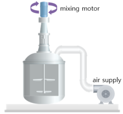
Figure 6. A schematic of TNT soil slurry reactor systems. The figure was redesigned to give better understandings based on the reference [36].
