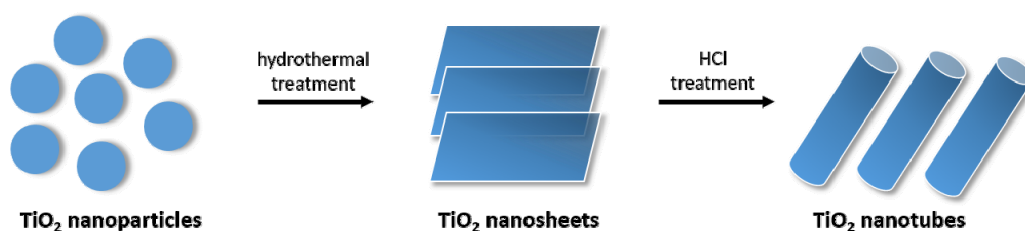
Figure 8. Schematic illustration for the synthesis procedure of TNT catalyst.
