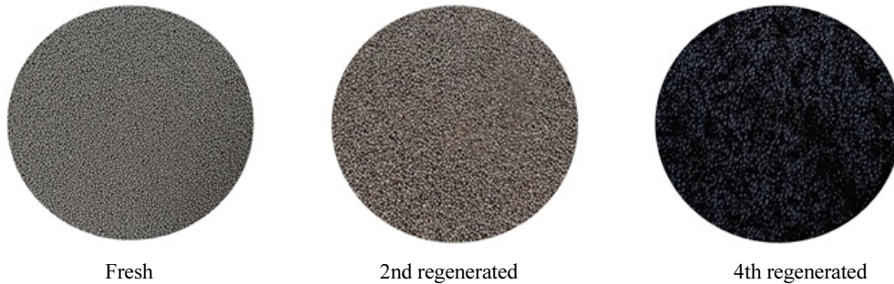
Figure 7. Images of fresh and regenerated Amberlyst-15 catalysts.
