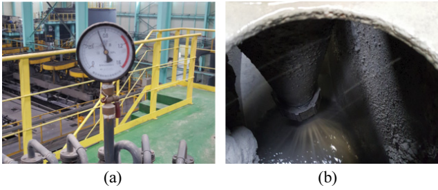
Figure 3. Photographs of hydro-cyclone in this study; (a): feed pressure, (b): under flow.
