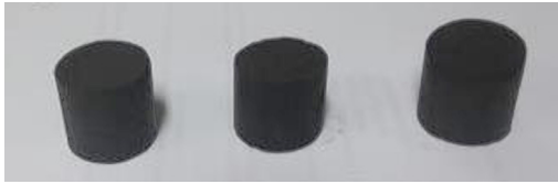
Figure 5. Pellets made by extrusion.
