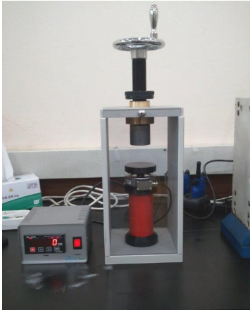
Figure 6. Compressive strength measuring device.
