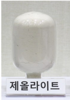
Figure 4. An image of syn-zeolite 4A type using coal waste.
