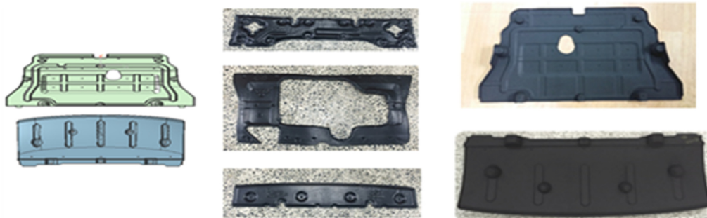
Figure 1. Under cover in engine room, (a) existing product, (b) uni-materialized product.
