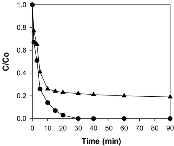
**Figure 2.** Correlations between the relative concentrations of 1,4-dioxane(●) and TOC(▲) observed during the reaction with 10 g copper wire and 200 mM H<sub>2</sub>O<sub>2</sub>.
