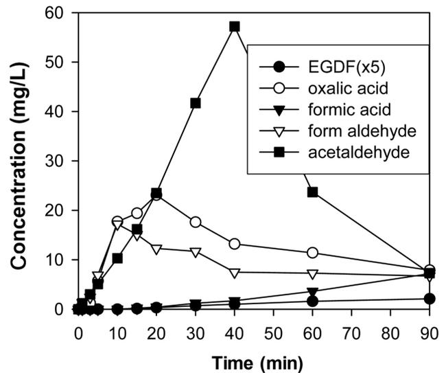
Figure 8. Concentration profiles of the main intermediates during the oxidation of 1,4-dioxane with 10 g Cu wire and 200 mM H<sub>2</sub>O<sub>2</sub>.
