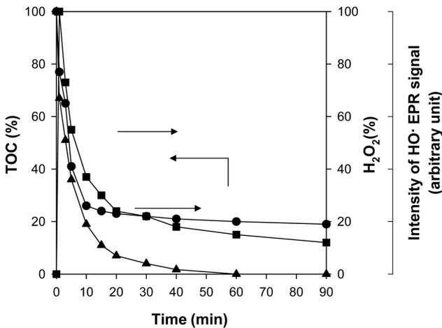
**Figure 3.** Correlation between TOC removal(●), H<sub>2</sub>O<sub>2</sub> consumption(▲) and HO· formation(■) during the catalytic wet peroxide oxidation of 1,4-dioxane with 10 g Cu wire and 200 mM H<sub>2</sub>O<sub>2</sub>.
