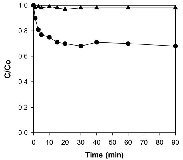
Figure 7. Time dependence of 1,4-dioxane(●) and TOC(▲) concentration during the reaction with 10 g Cu wire and 20 mM H<sub>2</sub>O<sub>2</sub>
