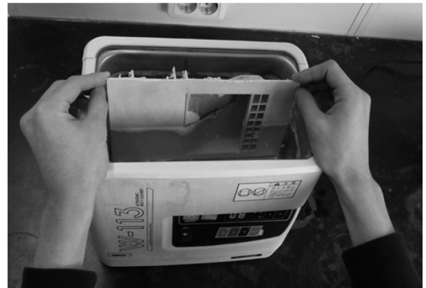
Figure 1. Ultrasonic cleaning test of laser copy machine parts with various cleaning agents.
