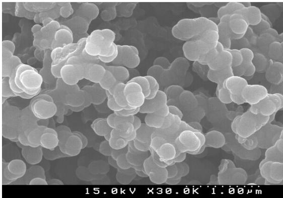
Fig. 10. SEM image of carbon black.( $\times 30,000$ )
